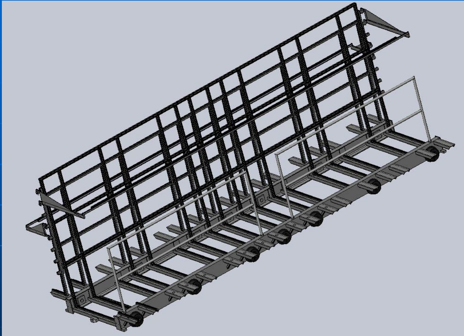
Chargierwagen (Fixed Charge cart, used for transport and storing of glass tables during sterilisation, for laminated glass production)
