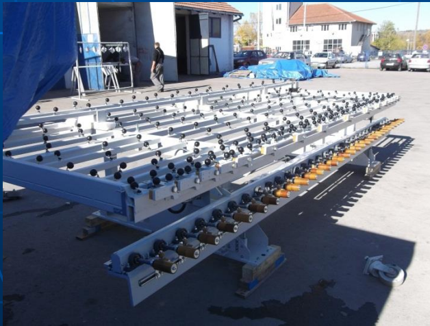
Lifting table with vertical rolls- hydraulic
