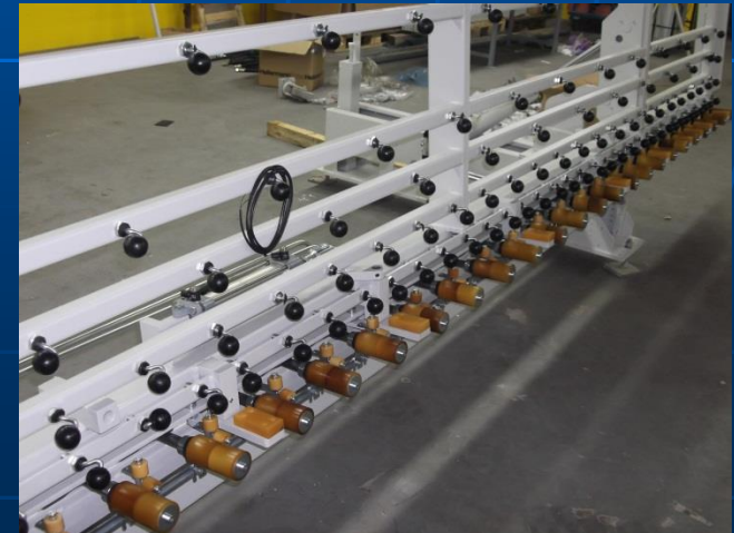
Lifting table with vertical rolls- hydraulic
